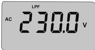
Fig 8.2 Low Pass Filter mode
